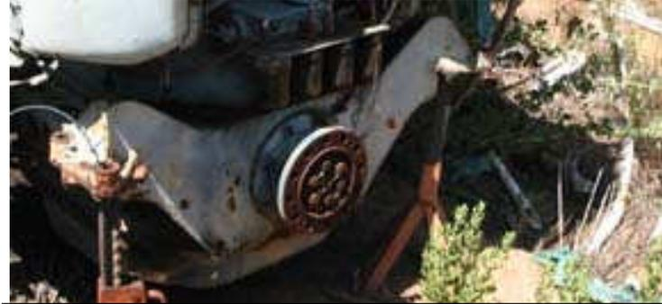
The bottom of the 16-A184 showing the horizontal output
